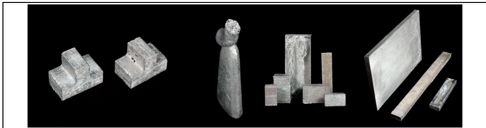
Fig. 14. 3D-parts of Al-alloy foams.
