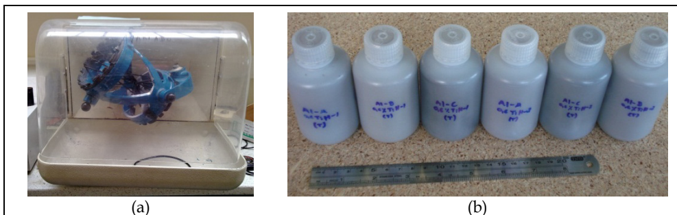
Fig. 5. (a) Turbula mixer used to mix the powders. (b) Powder mixtures.
