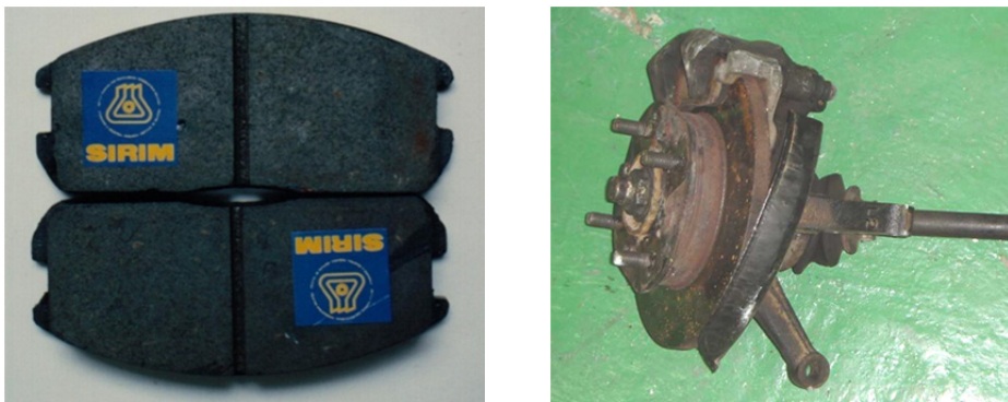
Fig. 2. Semi-metallic brake pad and front axle brake system
