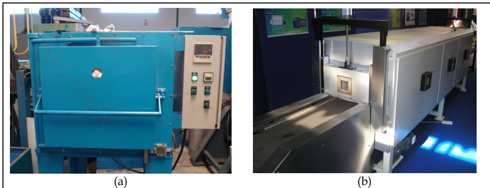
Fig. 13. Foaming furnaces. Batch chamber furnace (a). Continuous foaming furnace developed by this research team (b).
