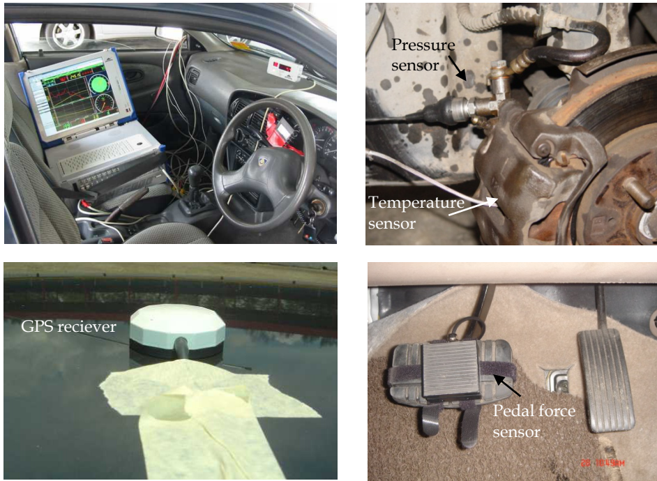
Fig. 3. Test equipment set-up; (a) Dewetron DEWE-5000 system, (b) pressure sensor and thermocouple, (c) GPS receiver installed on the roof (d) pedal force sensor.
