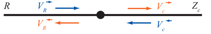
FIG. 15 (Color online) Semi-infinite transmission line of impedance Z_c terminated by a resistor R which is represented as a second semi-infinite transmission line.
