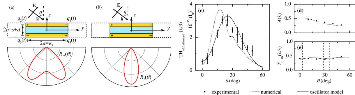
Fig. 1: (a), (b): parameters and far-field radiation pattern; (c): measured, simulated and modeled angular dependence of third harmonic for a fishnet structure at the magnetic resonance; (d), (e): measured and simulated linear angular dependence of absorption at fundamental wavelength and transmission at third harmonic wavelength, vertical lines in (e) corresponds to transmitted diffraction orders
