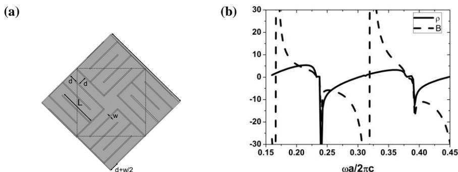
Fig. 1 (a) Structural unit cell in coiling-up space. Dashed-line encloses square unit cell of width  $a$ . (b) Effective density  $\rho$  and bulk modulus  $B$  of the metamaterial.
