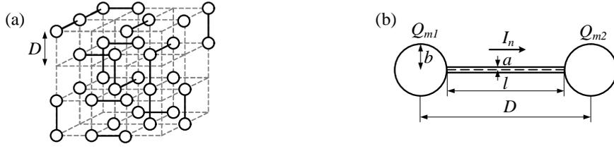
Fig. 1: (a) An example of 3-dimensional structure of conducting spheres connected by wires. Parameter  $D$  is the size of the cubic unit cells. (b) Parameter  $a$  is the radius and  $l$  is the length of the wire.  $b$  is the radius of the spheres. Current  $I$  and charges  $Q$  are on the surface of the wire and spheres, respectively.
