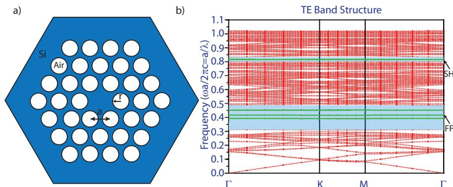
Fig. 1: a) Schematic of the photonic crystal cavity. b) Band structure of the photonic crystal obtained by using a  $5 \times 5$  supercell; bandgaps are denoted by using blue shaded colouring. Horizontal green lines indicate cavity modes.
