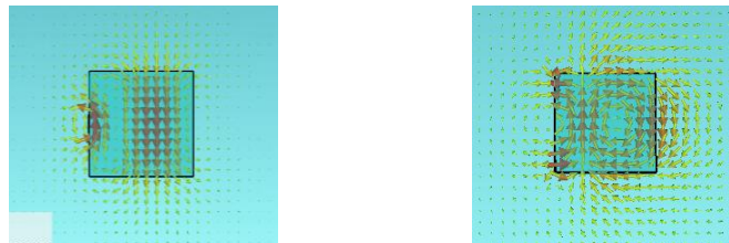
Fig. 2: Distribution of the magnetic (a) and electric (b) field components in case of magnetic resonance (first Mie resonance) of the dielectric cube.
