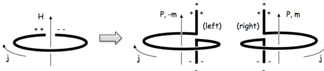
Fig. 1: Chirality by shape. Deforming a non-chiral single-ring SRR out of plane makes it chiral.
