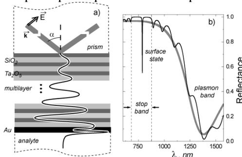
Fig. 1: (a) Geometry of analysis with a schematic distribution of the E-field for a resonant wave. (b) P-polarized reflection spectra of a 40-nm-thick Au layer (gray) and a PPhC sensor (black) terminated by the same Au layer. Spectra plotted in Fig. 1(b) were calculated for a PPhC of  $(\text{Ta}_2\text{O}_5/\text{SiO}_2)^{11}/\text{Au}$  at  $\alpha = 63.3^\circ$ ,  $D = 30$  nm.
