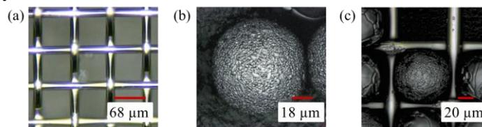
Fig. 1: Micrographs of (a) the metal-mesh, (b) TiO<sub>2</sub> sphere, and (c) composite structure.
