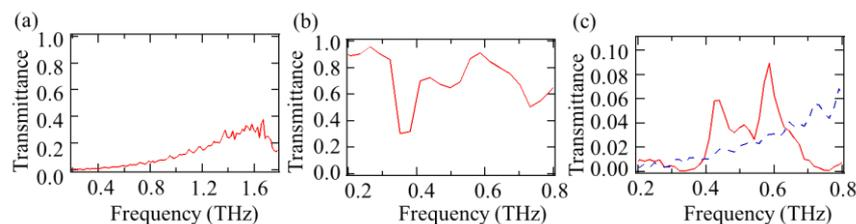
Fig. 2: Transmission spectra of (a) the metal-mesh, (b) TiO<sub>2</sub> spheres, and (c) composite structure. The dashed line in (c) is the transmission of a metal-mesh
