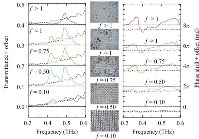
Fig. 3: Transmission and phase shift spectra of the composite of the  $\text{TiO}_2$  spheres and the metal-mesh for various ratios of the numbers of the  $\text{TiO}_2$  spheres to the opening of the metal-mesh  $f$ . The dashed lines indicate the metal-mesh for comparison. The dotted straight lines indicate the offset.
