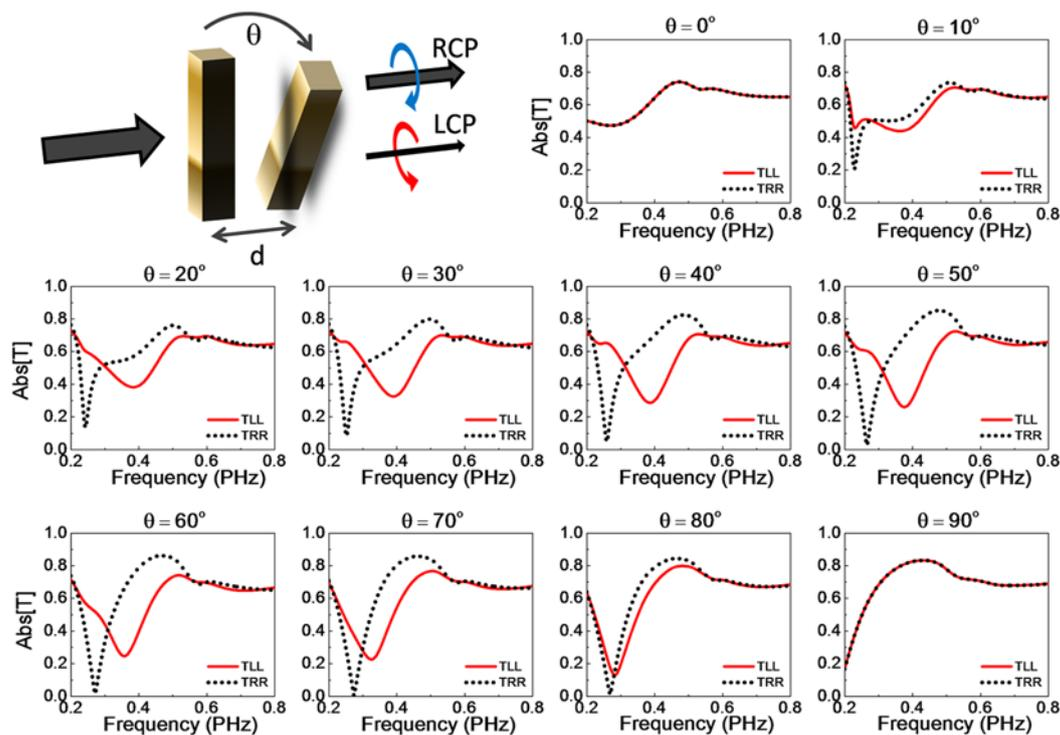
Fig. 1: The difference between transmission coefficients for right hand and left hand circular polarized light varying relative rotation angles, the inset shows the schematic configuration of the geometry under analysis.
