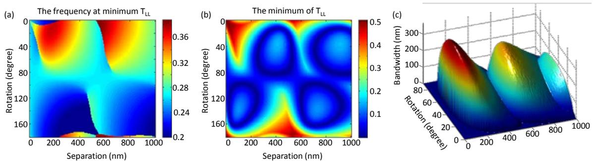
Fig. 3: (a) Color map of the frequency of minimum  $T_{LL}$  for a pair of metasurfaces consisting of gold nanorods with varying separations distances from 0 nm to 1000 nm and a rotation angle between  $0^\circ$  and  $180^\circ$ . (b) The difference between  $T_{LL}$  and  $T_{RR}$  with varying separation distances. (c) 3D view of the bandwidth variation with separation and rotation angle.
