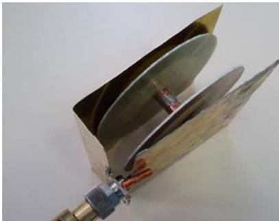
Fig. 6: Scaled DB unit cell placed inside parallel-plate capacitor.
