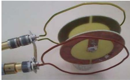
Fig. 4: Scaled DB unit cell placed between two loop antennas.
