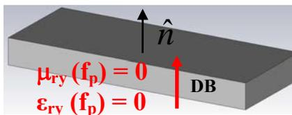
Fig. 1: DB material with zero-permittivity and zero-permeability in direction normal to the surface.
