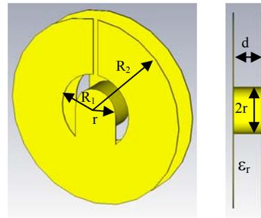
Fig. 2: Simplified composite unit cell that simultaneously behaves as MNZ and ENZ particle. Left: isometric view, Right: side view.  $r=0,7\text{mm}$ ,  $R_1=1\text{mm}$ ,  $R_2=2,5\text{mm}$ ,  $d=0,7\text{mm}$ ,  $\epsilon_r=2,6$ .
