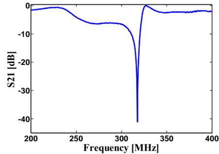
Fig. 5: Measured transmission coefficient reveals zero-permeability at frequency 318 MHz.
