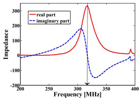
Fig. 7: Setup impedance calculated from measured reflection coefficient. Zero-permittivity is achieved at frequency 318 MHz.
