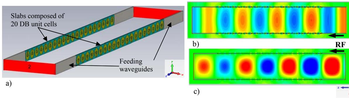
Fig. 3: **a)** Waveguide structure with walls made of DB slabs. **b)** Magnetic field distribution inside the waveguide, while PMC boundary conditions were applied in y-direction. **c)** Electric field distribution inside the waveguide, while PEC boundary conditions were applied in y-direction.
