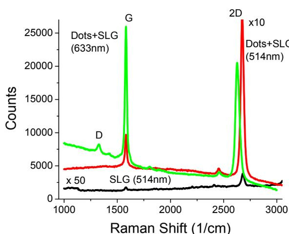
Fig. 1: The experimental enhancements for main Raman bands of graphene layer on top of Au nanodots.
