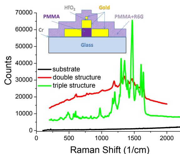
Fig. 2: The Raman spectra (laser power  $\sim 200\mu\text{W}$ ,  $\tau\approx 60\text{s}$ ). Inset: schematic of the cross-section of the structure with a coating of PMMA/dye.
