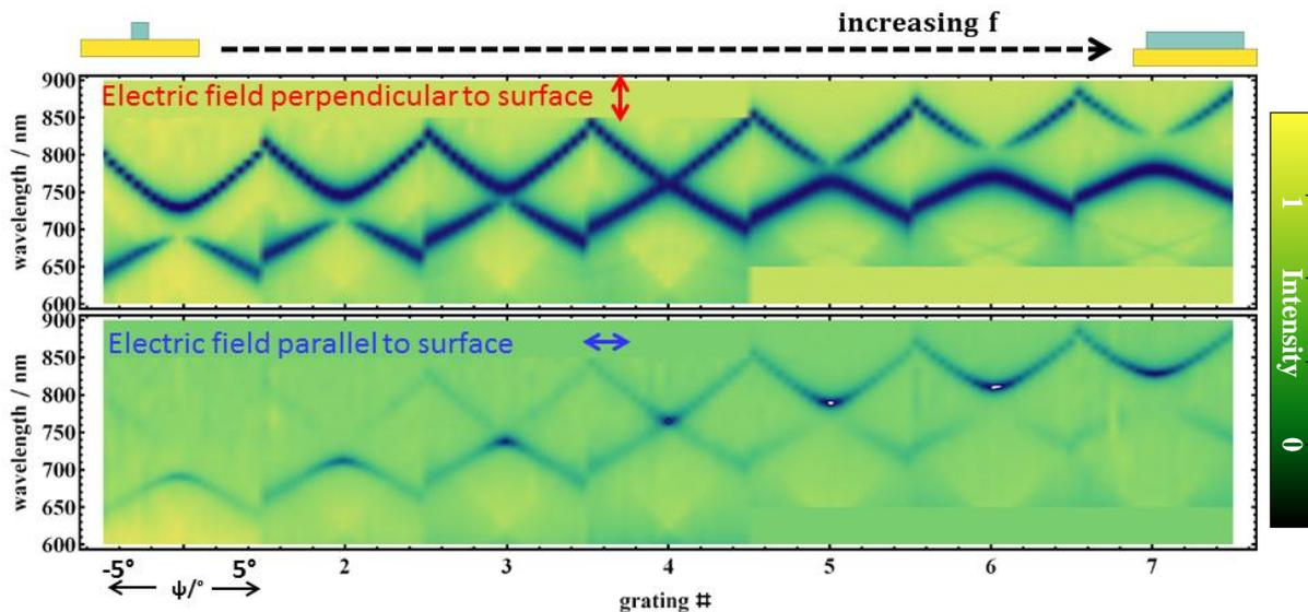
Fig. 2: Far field reflection measurements scanning the dispersion around the bandgap for gratings with varying filling factor  $f$ . The scaled reflection intensity is shown color coded. The bandgap shifts to lower energies with increasing  $f$  (I) and changes in size  $\Delta E$  (II). Another gap in  $k$ -direction occurs in different branches depending on the polarization used for excitation (III).
