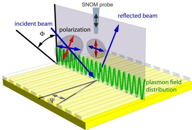
Fig. 1: Illumination settings used to excite plasmons in our setup.
