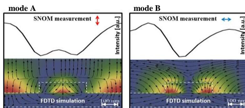
Fig. 3: Extract of our near field SNOM measurements for each polarization at  $\psi = 0$ . In accordance to FDTD simulations we clearly detect different mode patterns (mode A and B) for each polarization setting. Electric field directions were extracted from the simulations (black arrows).
