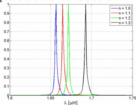
Fig. 3: Spectra of the resonant modes of the hexagonal PhC cavity for different values of the refractive indices of the central hole.
