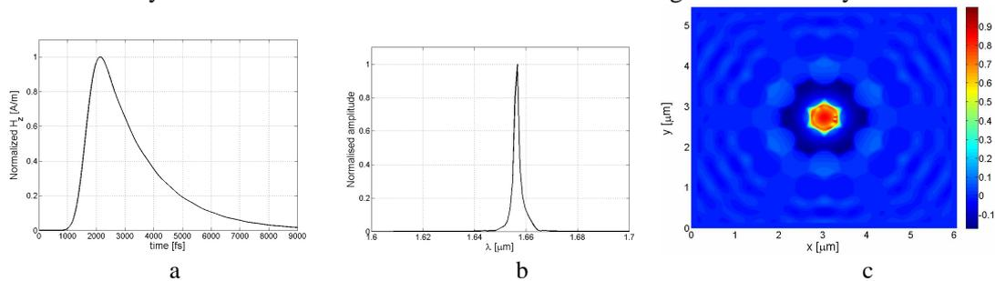
Fig. 2: a) Envelope of the time domain evolution of the resonant mode; b) spectrum of the resonant mode; c) field profile of the resonant mode
