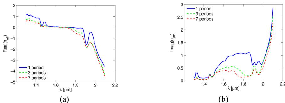
Fig. 3: Spectral dependences of the real (a) and imaginary (b) parts of the effective refractive index of fishnet structures under consideration, with the dependence on the number of MIM periods as the parameter.
