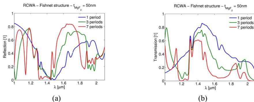
Fig. 2: Reflection (a) and transmission (b) intensity spectra of the fishnet structure, with the dependence on the number of MIM periods as the parameter.
