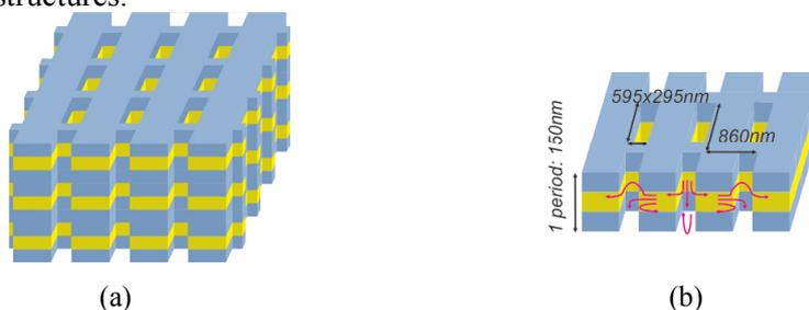
Fig. 1: (a) Example of fishnet metamaterial structure consisting of several MIM layer periods (typically of 150nm thickness), (b) detailed vertical 1 period cut revealing interaction processes inside fishnet structure.
