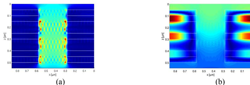
Fig. 4: Demonstration of the calculated field profiles within 3 MIM period fishnet structure: (a) absolute value of the  $E_x$  and (b)  $H_y$  fields ( $\lambda=1.78\mu\text{m}$ ).
