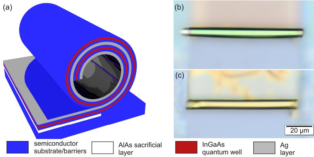
Fig. 1: (a) Sketch of a rolled-up microtube whose walls represents a rolled-up metamaterial consisting of Ag (13 nm) and (AlIn)GaAs (51 nm) containing an optically active quantum well (7 nm). (b,c) Optical micrographs of metamaterials which are rolled-up three (b) and two (c) times, respectively.
