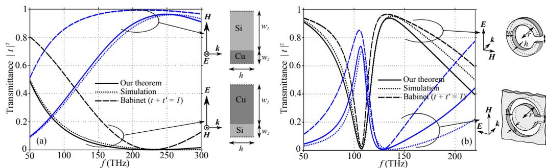
Fig. 2: Left: transmission through two complementary 1D diffraction screens made of alternating layers of copper and silicon (unit cells shown aside). Dimensions are  $w_1 = 50$  nm,  $w_2 = 10$  nm and  $h = 25$  nm. Right: transmission through complementary silver SRR and CSRR screens with  $r = 100$  nm,  $g = 10$  nm,  $w = 30$  nm and  $h = 60$  nm. Periodicity is 250 nm.
