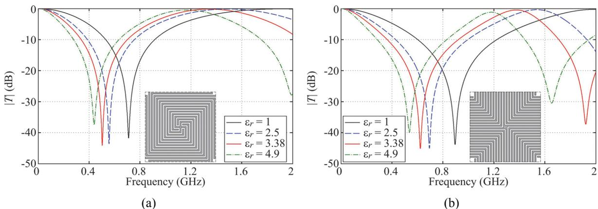
Fig. 1: Transmittance of the intertwined quadrifilar spiral (a) and Brigid's cross (b) arrays on dielectric substrate with permittivities  $\epsilon_r = 1, 2.5, 3.38, 4.9$ . The square unit cells shown in the inserts have size  $p = 10.8$  mm, and the widths of strips ( $s$ ) and gaps ( $g$ ) are  $s=g=0.2$  mm, and the conductor thickness is  $17.5 \mu\text{m}$ .
