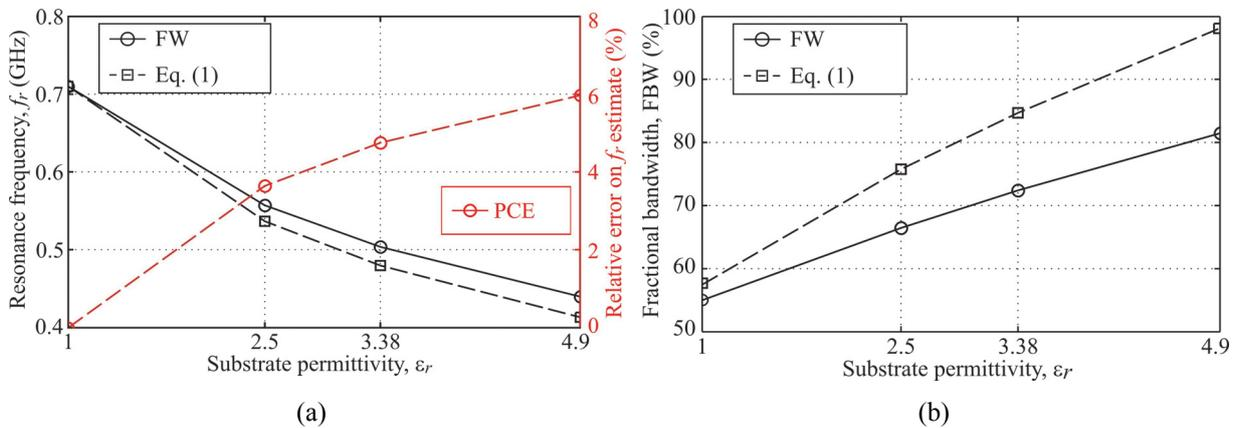
Fig. 2: Resonance frequencies (a) and FBW (b) for the intertwined quadrifilar spiral arrays on dielectric substrates with variable permittivity  $\epsilon_r = 1, 2.5, 3.38, 4.9$ . Data from full-wave (FW) simulations in Fig. 1 are compared with the values predicted by (1). Lines provide an eye-guide only.
