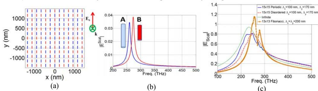
Fig. 3: (a)  $13 \times 13$  Fibonacci Array, (b) Scattering performance of the **A** and **B** nanorods, (c) Optical performance of finite periodic, disordered, infinite and Fibonacci arrays.
