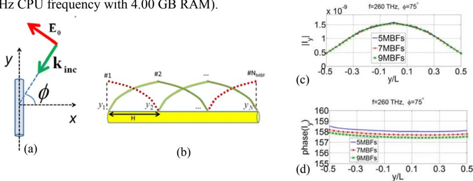
Fig. 1: (a) A plasmonic nanorod illuminated by an oblique planewave, (b) Discretization of the polarization current, (c) Magnitude and (d) Phase of the polarization for  $\phi=75^\circ$  and  $f=260$  THz
