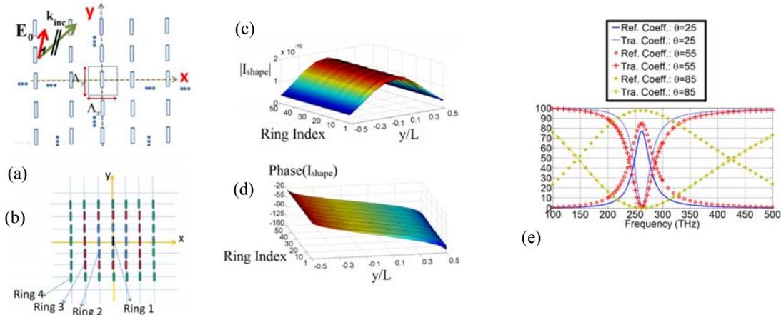
Fig. 2: (a) Array illuminated by an oblique wave, (b) Ring definition, (c) Magnitude and (d) Phase of the macro-CBF versus ring index and length of the nanorod, (e) Reflection and transmission coefficient for three different values of  $\theta = 25^\circ, 55^\circ, \text{ and } 85^\circ$ .
