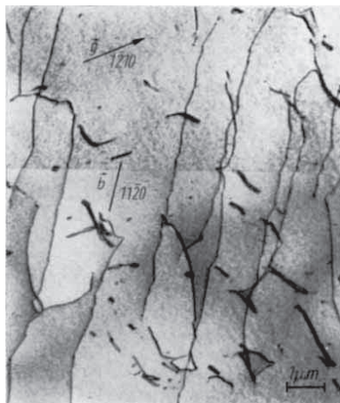
Fig. 3. Examples of numerous cusps in the dislocations predominantly of screw character associated with visible obstacles. b = 1/3 [11\bar{2}0]
