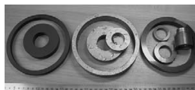
Fig. 1. Sequence of structural SiC ceramics production: (left) SiC–carbon blanks, (middle) siliconized blanks, and (right) final articles after mechanical treatment.
