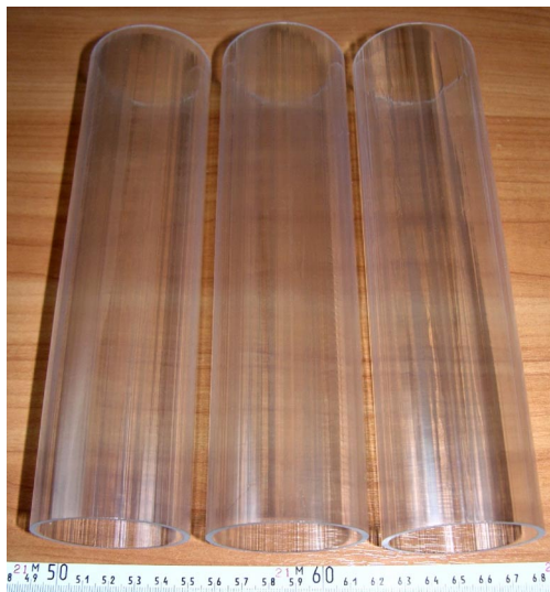
Fig. 10 Sapphire tubes of 55 mm in external diameter grown with automated EFG (Stepanov) technique. (Online color at www.crt-journal.org )
